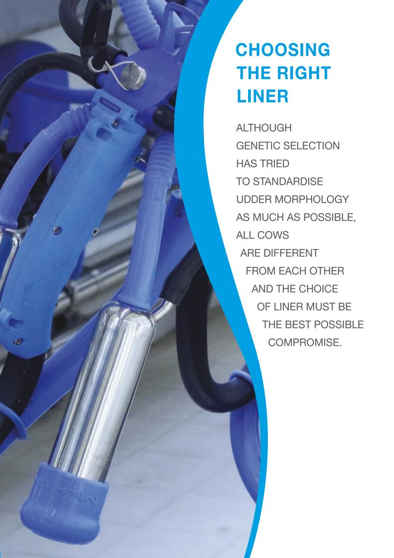
When choosing the right liner, you should not only take into account the shape and size of the teats and breed of your cows, but also the **type of claw** on which the liners will fit. The **liner material** should also be taken into account.
